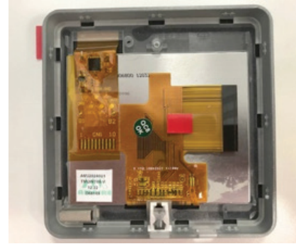
Combining a touch FPC and TFT FPC into a single custom FPC.
